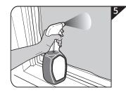
Spray film surface with water. Using a squeegee, remove moisture starting from the centre out to the edges.
