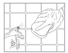
Clean the tiles thoroughly to remove any grease or dirt, then leave to dry.
