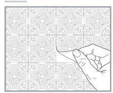
Using a dry cloth, smooth the sticker into position, pushing any bubbles out to the edges. Ensure all 4 sides are stuck down firmly.
